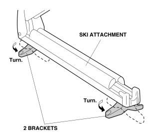
4. Using a wrench, install the ski attachment to the front crossbar with four bolts, four collars, and two brackets.
